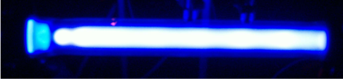
Figure 8: 1 Torr, 30 mA Argon Discharge
